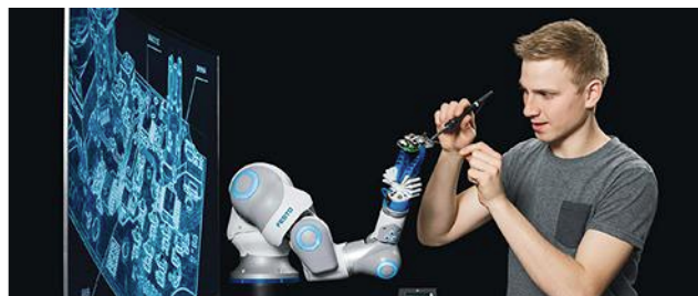
4. Festo's BionicCobot is a pneumatic lightweight robot that can work in close quarters with humans.
