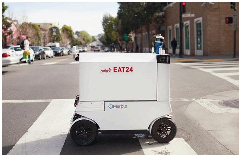
1. Marble's robot, controlled by an Nvidia Jetson TX1, delivers food in San Francisco that was ordered using a Yelp Eat24 app.
